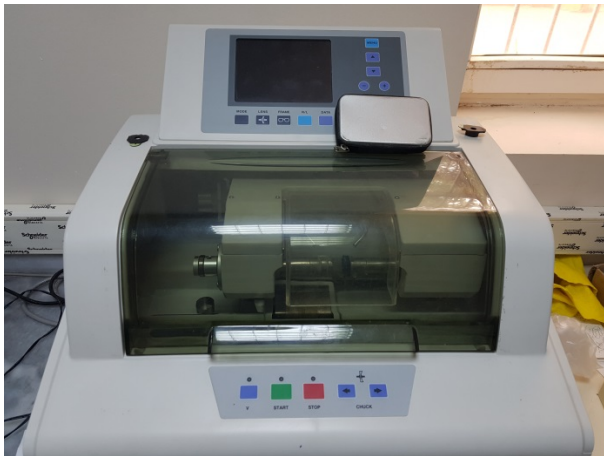
Figure-5 Automatic glass cutting machine.
